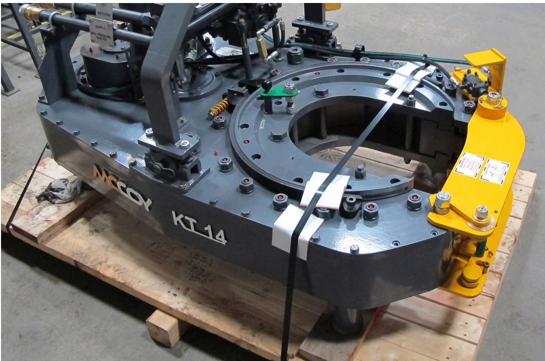
Illustration 5.10.2: Shipping Instructions - Strapping to Pallet
