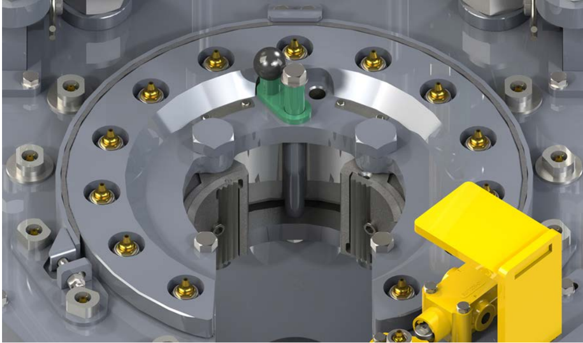
Illustration 4.1.2: Setting Backing Pin To “Make-up” Position
