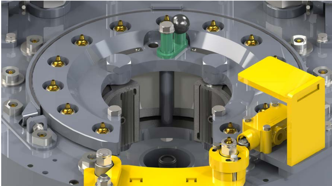
Illustration 4.1.3: Backing Pin Set To “Break-Out” Position
