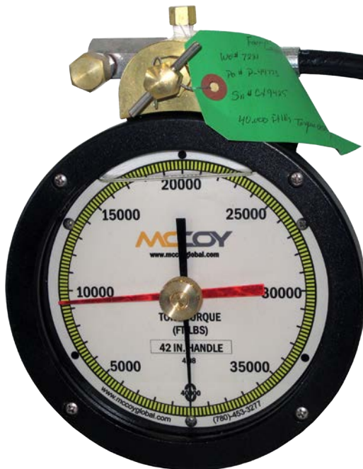
Illustration 8.0.1: Torque Gauge (For Illustration Purposes Only)
