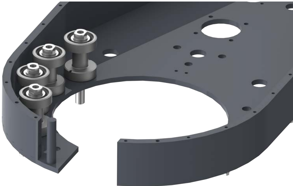
Illustration 5.9.1: Tong Assembly - Initial Support Roller Installation
