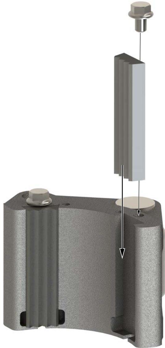
ILLUSTRATION 2.F.2: KT5500 STANDARD JAW DIE REMOVAL
