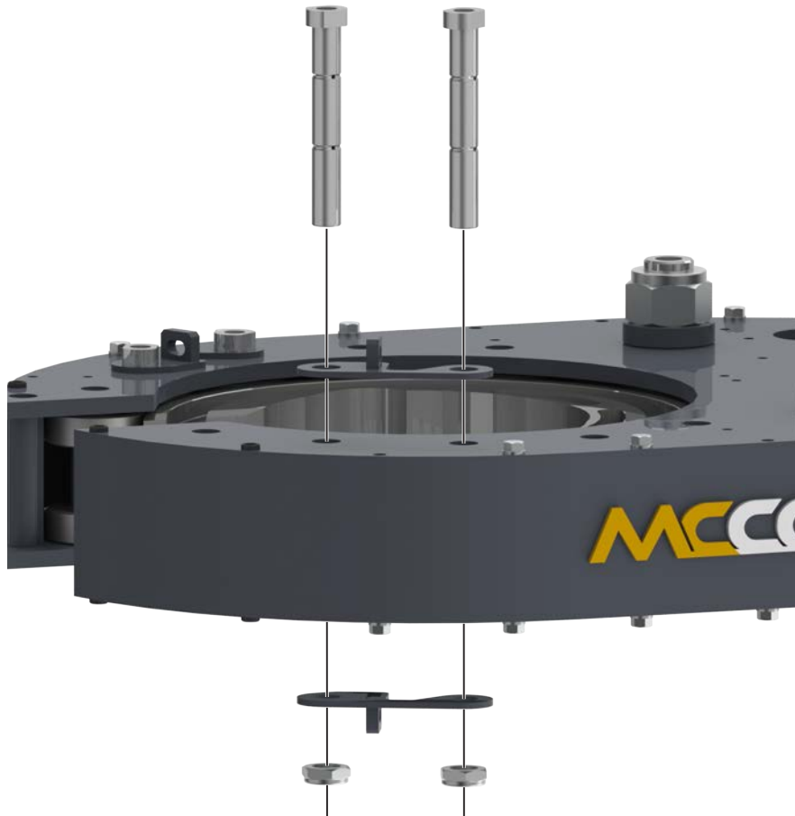
ILLUSTRATION 4.I.5: TONG ASSEMBLY - BRAKE BAND WELDMENT INSTALLATION
