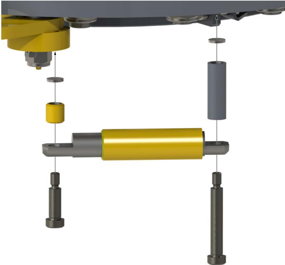
ILLUSTRATION 4.I.11: TONG ASSEMBLY - DOOR STOP SPRING CYLINDER INSTALLATION
