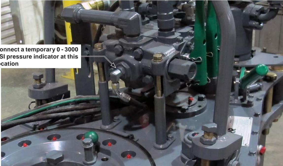
ILLUSTRATION 5.B.1: RELIEF VALVE TROUBLESHOOTING - TEMPORARY GAUGE INSTALLATION
