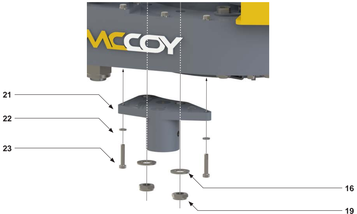
ILLUSTRATION 6.39: FRONT LEG WELDMENT INSTALLATION
