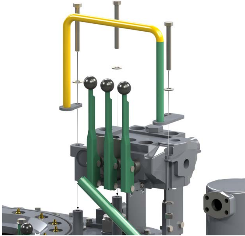
ILLUSTRATION 4.1.12: TONG ASSEMBLY - VALVE ASSEMBLY INSTALLATION
