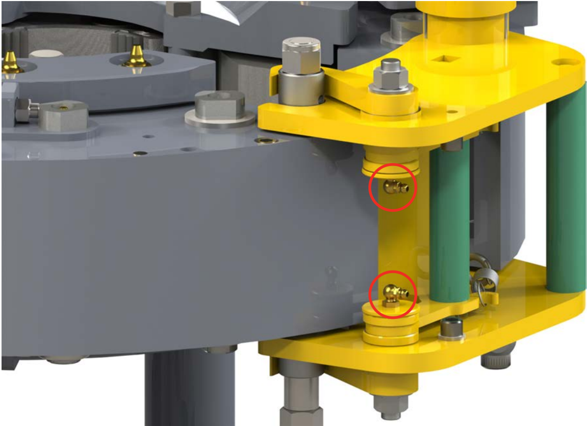
ILLUSTRATION 4.E.10: DOOR LATCH BUSHING LUBRICATION
