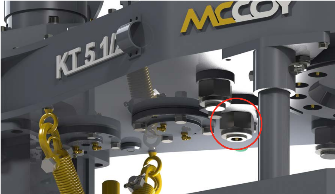
ILLUSTRATION 3.D.4: PINION IDLER BEARING LUBRICATION
