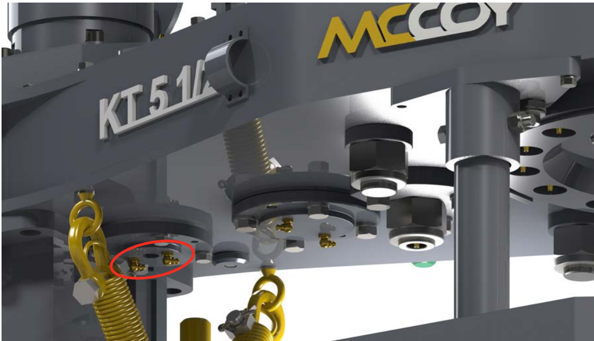
ILLUSTRATION 4.E.7: CLUTCH BEARING LUBRICATION
