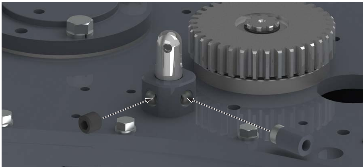
ILLUSTRATION 4.1.4: TONG ASSEMBLY - TOP SHIFTER BUSHING INSTALLATION
