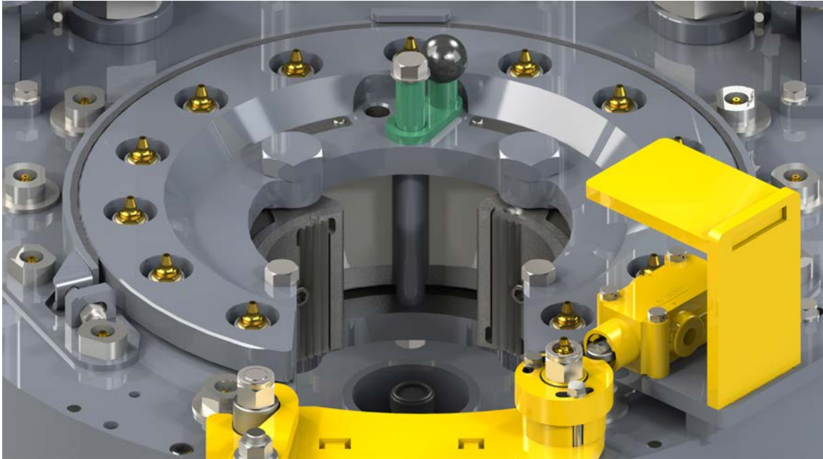
ILLUSTRATION 3.B.4: BACKING PIN CONFIGURED FOR “MAKE-UP” OPERATIONS
