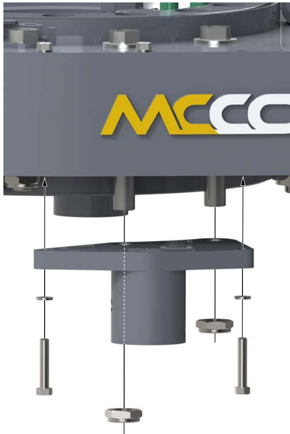
ILLUSTRATION 4.1.6: TONG ASSEMBLY - FRONT LEG MOUNT WELDMENT INSTALLATION
