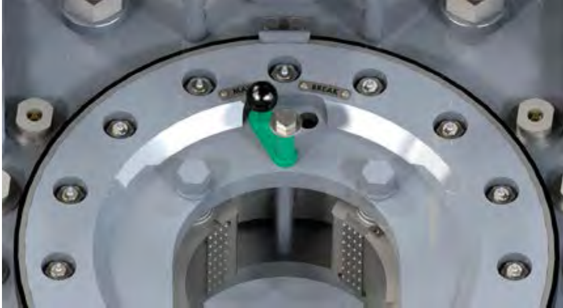
Illustration 4.1.2: Setting Backing Pin To “Make-up” Position
