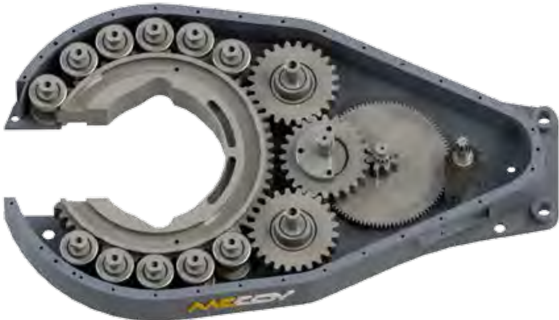
Illustration 5.9.2: Tong Assembly - Gear Assembly Positioning
