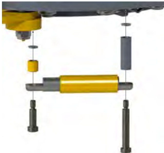
Illustration 5.9.10: Tong Assembly - Door Spring Stop Cylinder Installation
