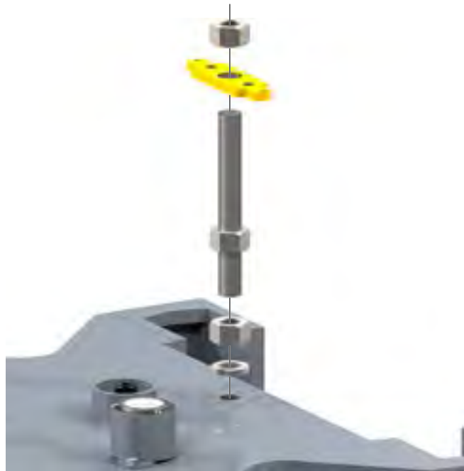
Illustration 5.9.11: Tong Assembly - Rear Backup Spring Support Bracket Installation
