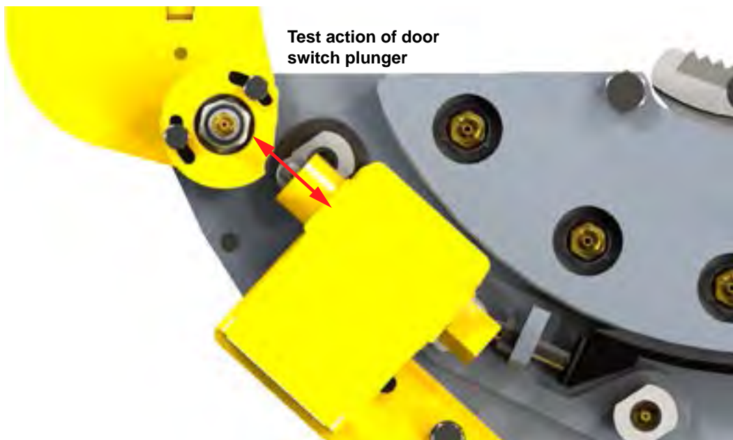
Illustration 5.6.4: Door Switch Adjustment 02
