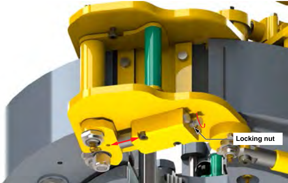
Illustration 5.6.7: Door Latch Adjustment 02
