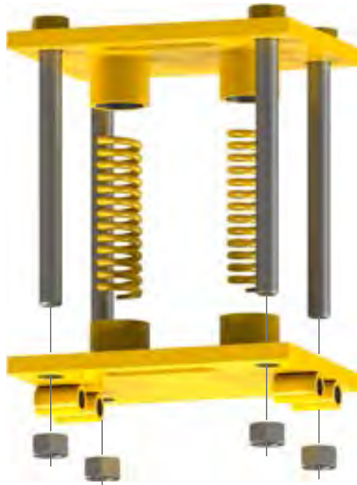
Illustration 5.9.12: Rear Leg Spring Support Installation (Model 80-0615-14)
