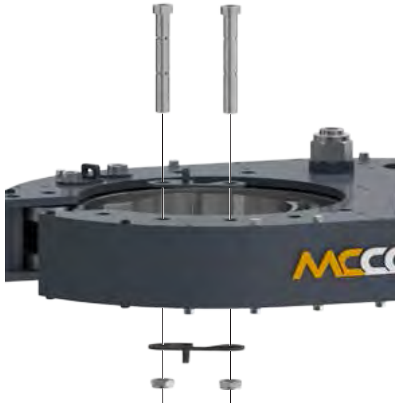
Illustration 5.9.4: Tong Assembly - Brake Band Coincidental Roller Shaft Installation
