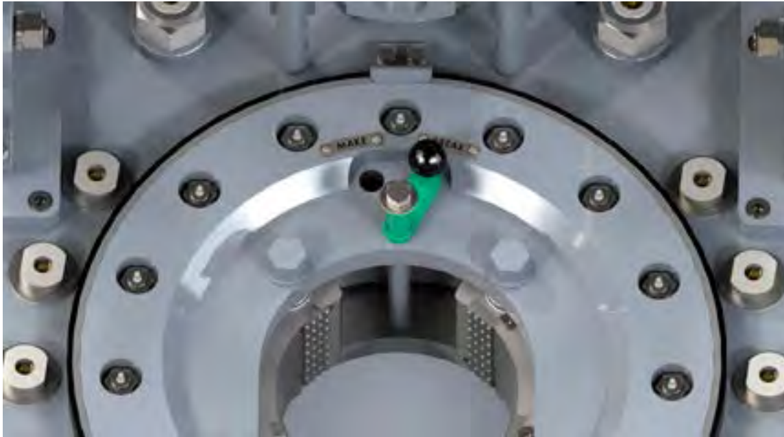
Illustration 4.1.3: Backing Pin Set To “Break-Out” Position
