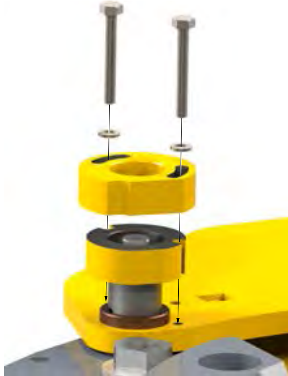
Illustration 5.9.9: Tong Assembly - Door Switch Cam Installation
