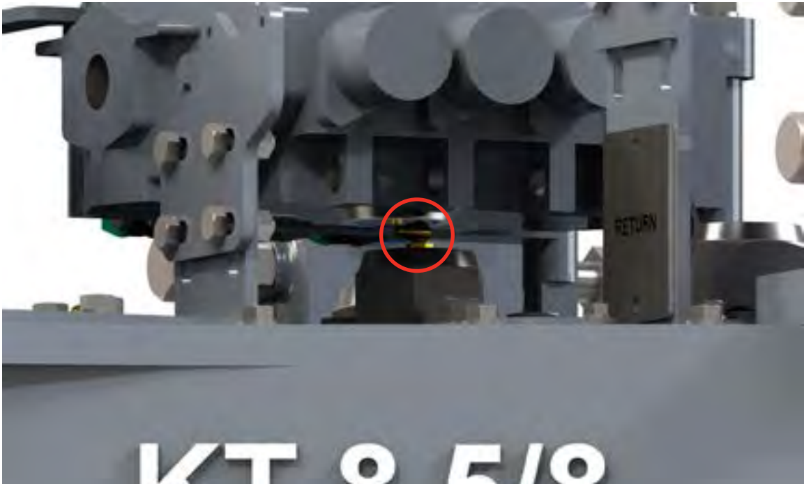
Illustration 5.5.4: Pinion Idler Lubrication Point
