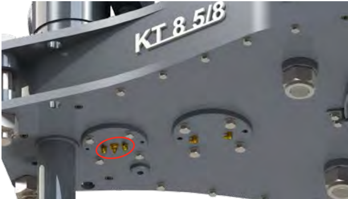
Illustration 5.5.6: Clutch Lubrication Points
