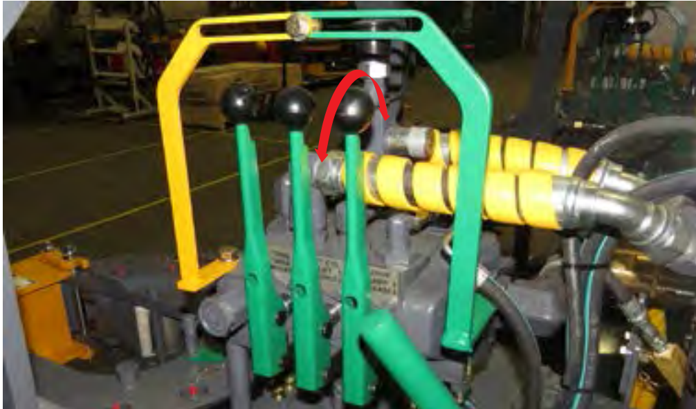
Illustration 4.0.3: Backup Control Valve
