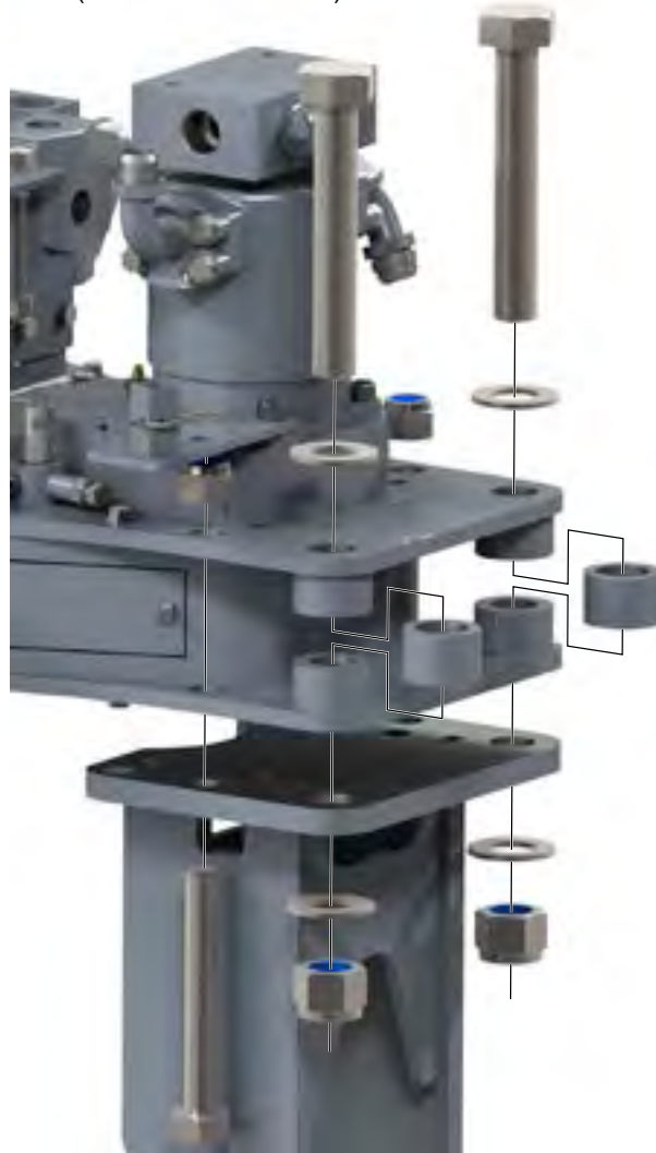
Illustration 5.9.13: Tong Assembly - Rear Leg Installation
