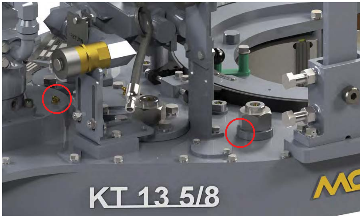
Illustration 5.5.10: Motor Mount Lubrication
