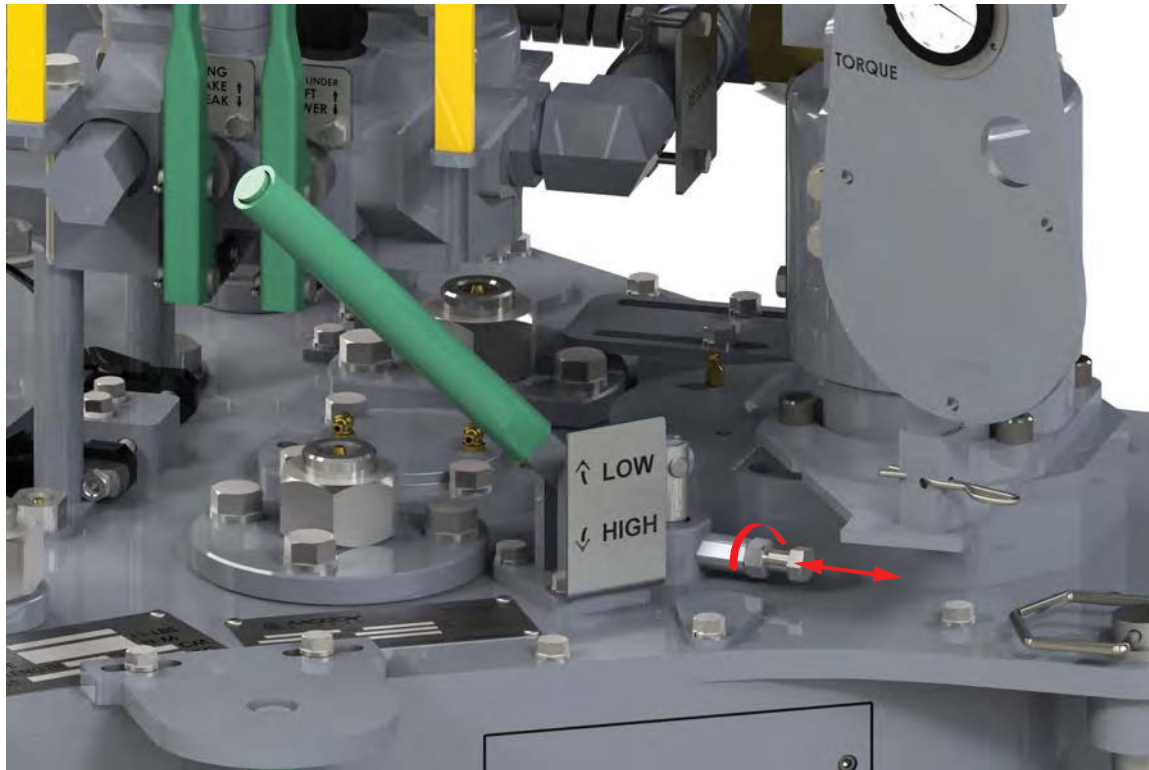
Illustration 5.6.6: Shifter Detent Force Adjustment
