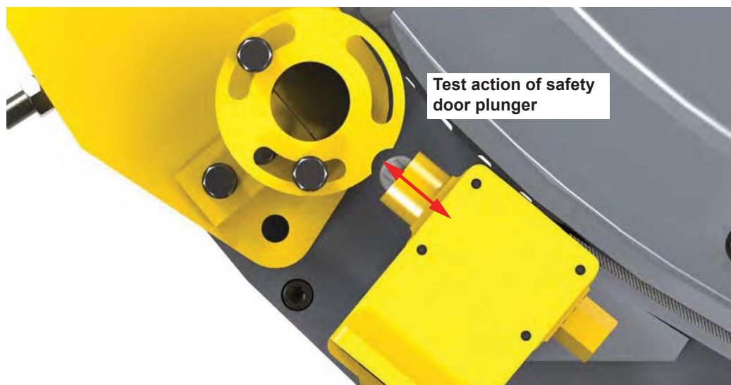
Illustration 5.6.8: Door Switch Adjustment 02
