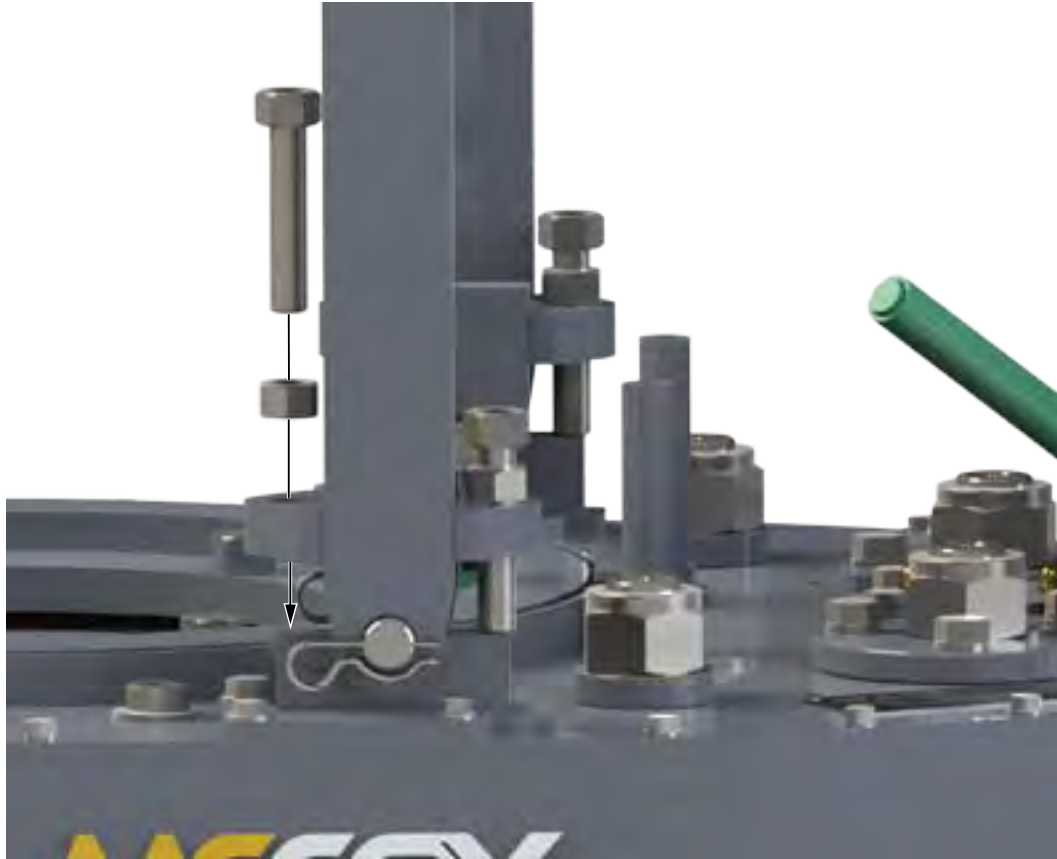
ILLUSTRATION 3.1.10: TONG ASSEMBLY - LEVELING BOLT INSTALLATION
