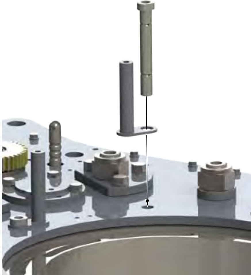
ILLUSTRATION 3.1.5: TONG ASSEMBLY - SUPPORT ROLLER INSTALLATION 02
