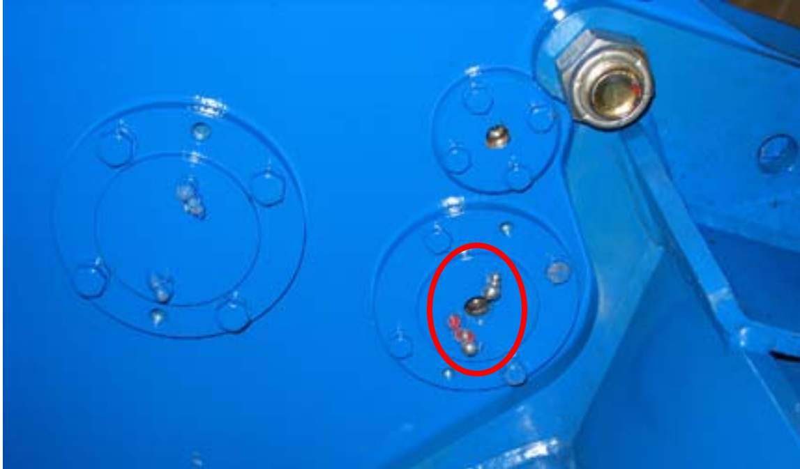
ILLUSTRATION 3.E.8: CLUTCH SHAFT LUBRICATION
