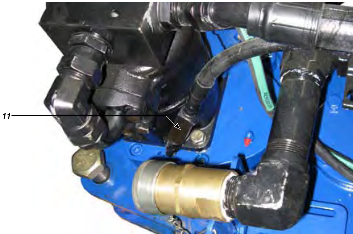
ILLUSTRATION 2.E.7: KT13625 TONG & FARR® BACKUP HYDRAULIC COMPONENT ID 03
