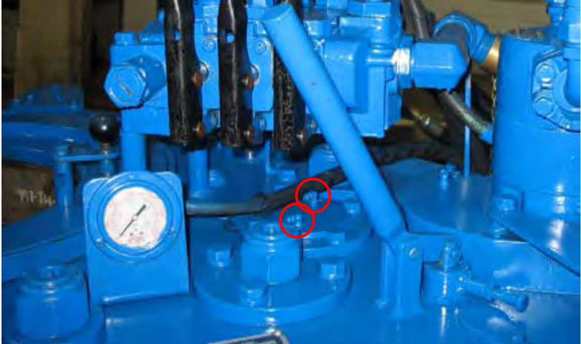
ILLUSTRATION 3.E.6: PINION LUBRICATION TOP PLATE
