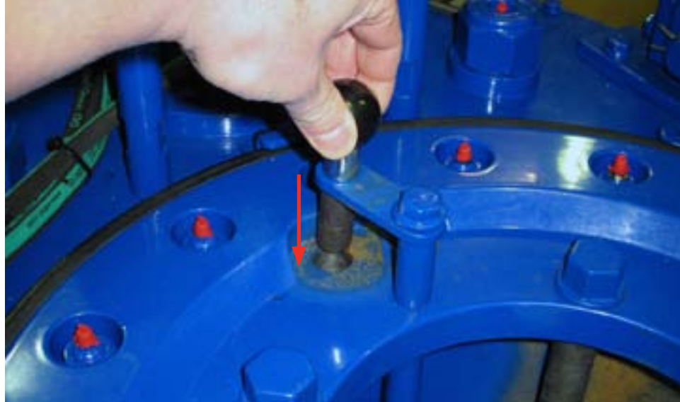
ILLUSTRATION 2.J.2: SETTING BACKING PIN TO "MAKE-UP" POSITION
