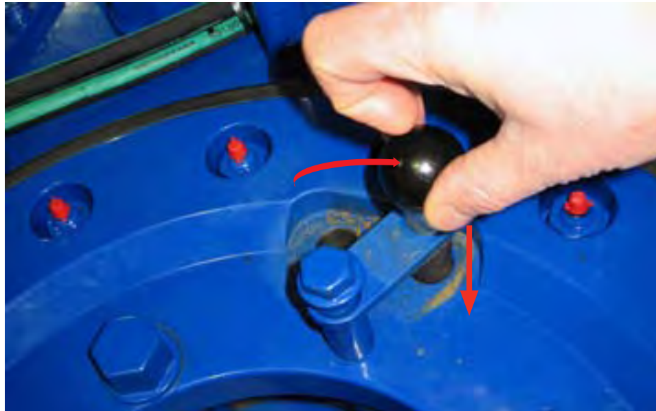
ILLUSTRATION 2.J.12: SETTING BACKING PIN TO BREAK-OUT POSITION
