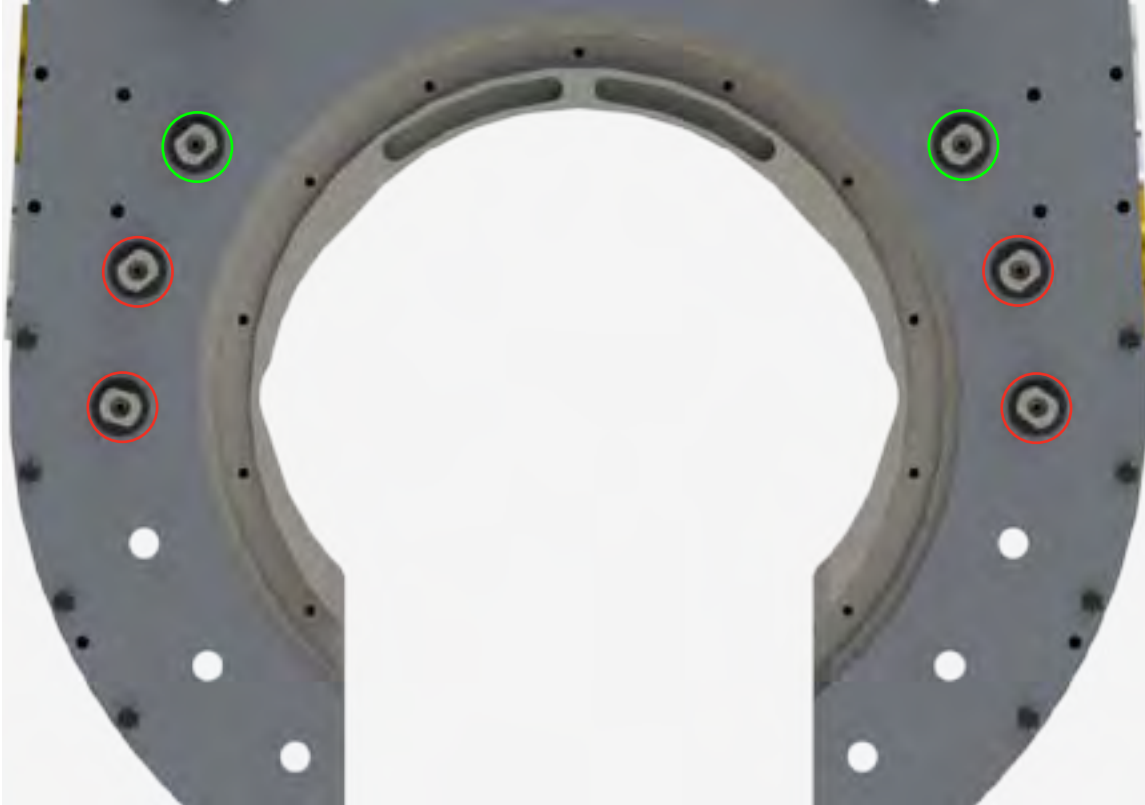
ILLUSTRATION 3.1.4: TONG ASSEMBLY - SUPPORT ROLLER INSTALLATION 01
