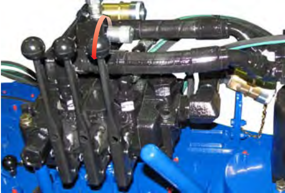
ILLUSTRATION 2.J.10: USING BACKUP CONTROL TO RELEASE BACKUP JAWS
