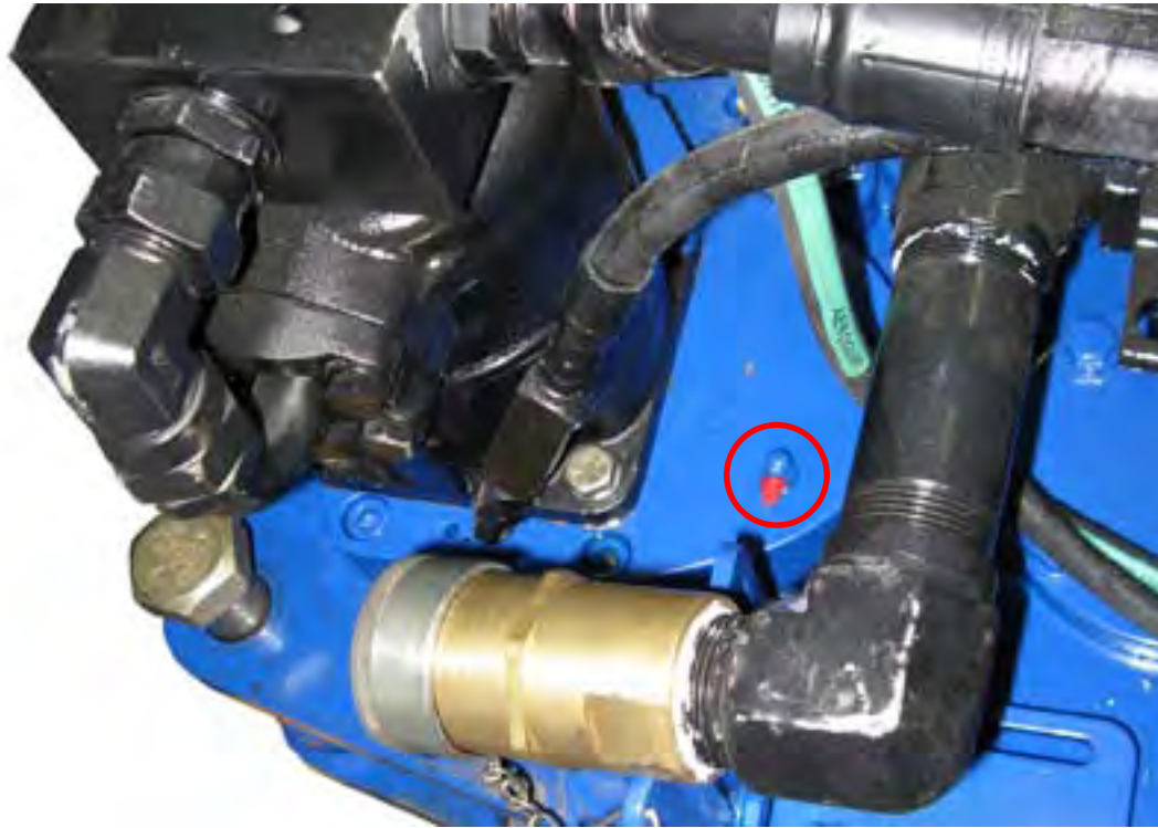
ILLUSTRATION 3.E.10: MOTOR MOUNT LUBRICATION
