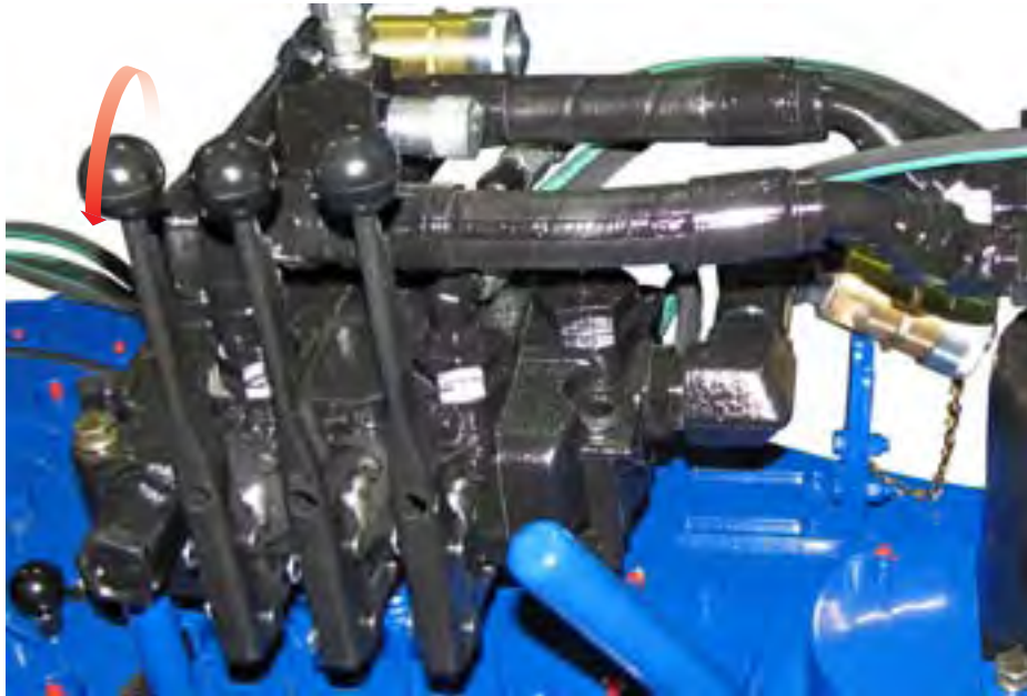
ILLUSTRATION 2.J.14: USING MOTOR CONTROL TO RELEASE JAWS IN "BREAK OUT" MODE
