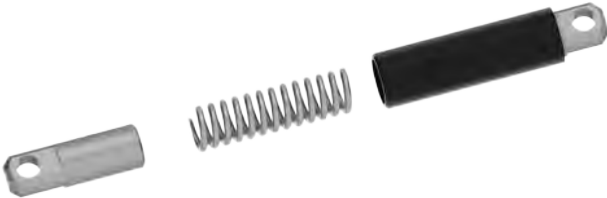
ILLUSTRATION 3.E.12: DOOR STOP SPRING LUBRICATION
