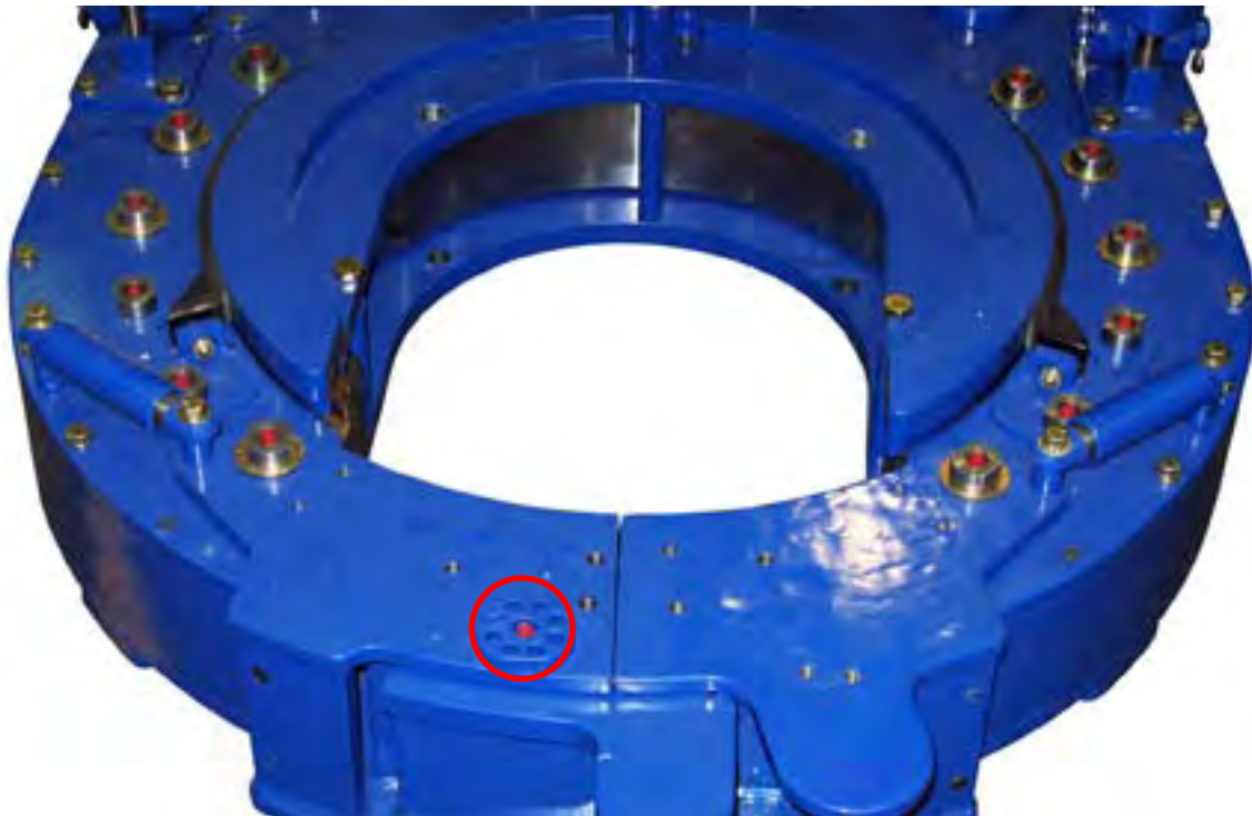
ILLUSTRATION 3.E.11: DOOR LATCH CAM LUBRICATION
