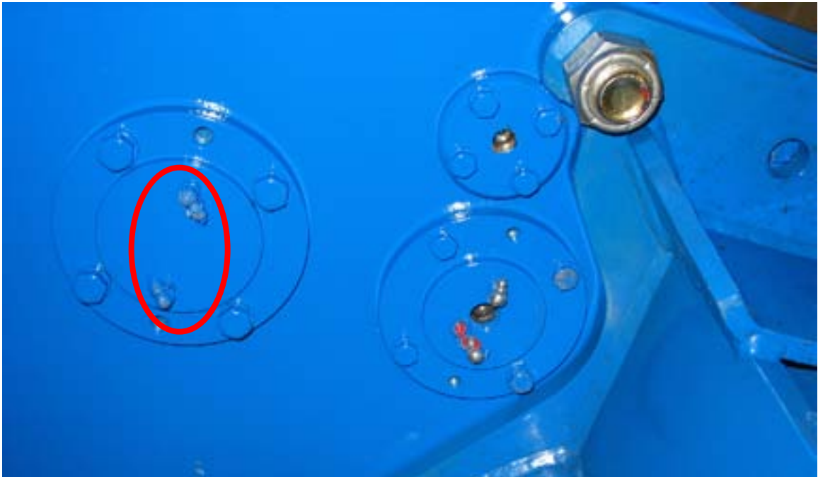
ILLUSTRATION 3.E.7: PINION LUBRICATION BOTTOM PLATE
