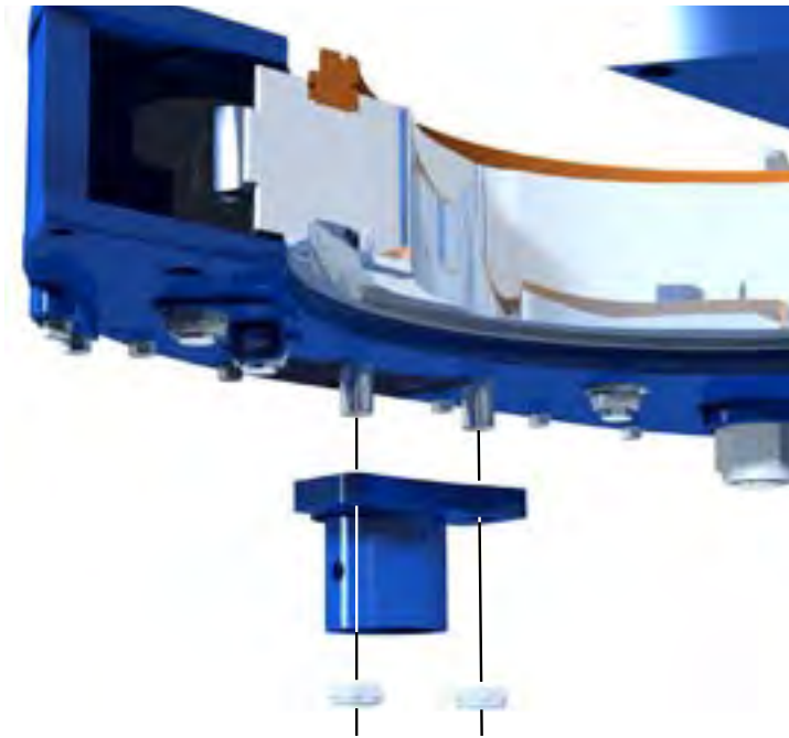
ILLUSTRATION 3.1.8: TONG ASSEMBLY - FRONT LEG MOUNT WELDMENT INSTALLATION
