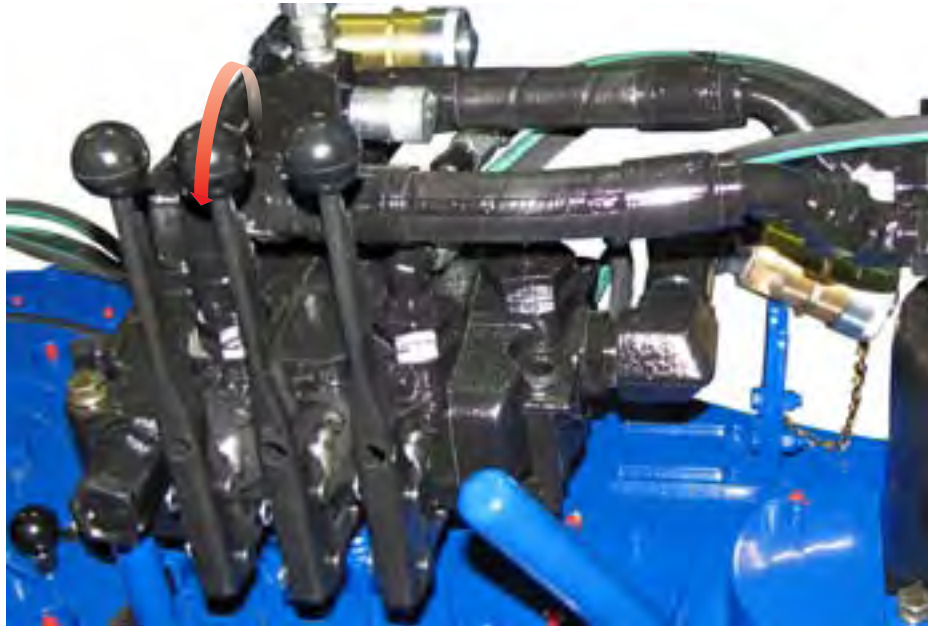
ILLUSTRATION 2.J.6: LIFT CYLINDER CONTROL - RAISE (NON CE-MARKED TONGS)
