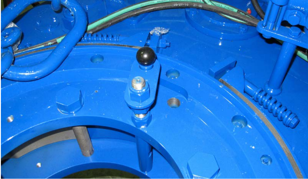
Illustration 2.1.2: Backing Pin Set To “Make-up” Position
