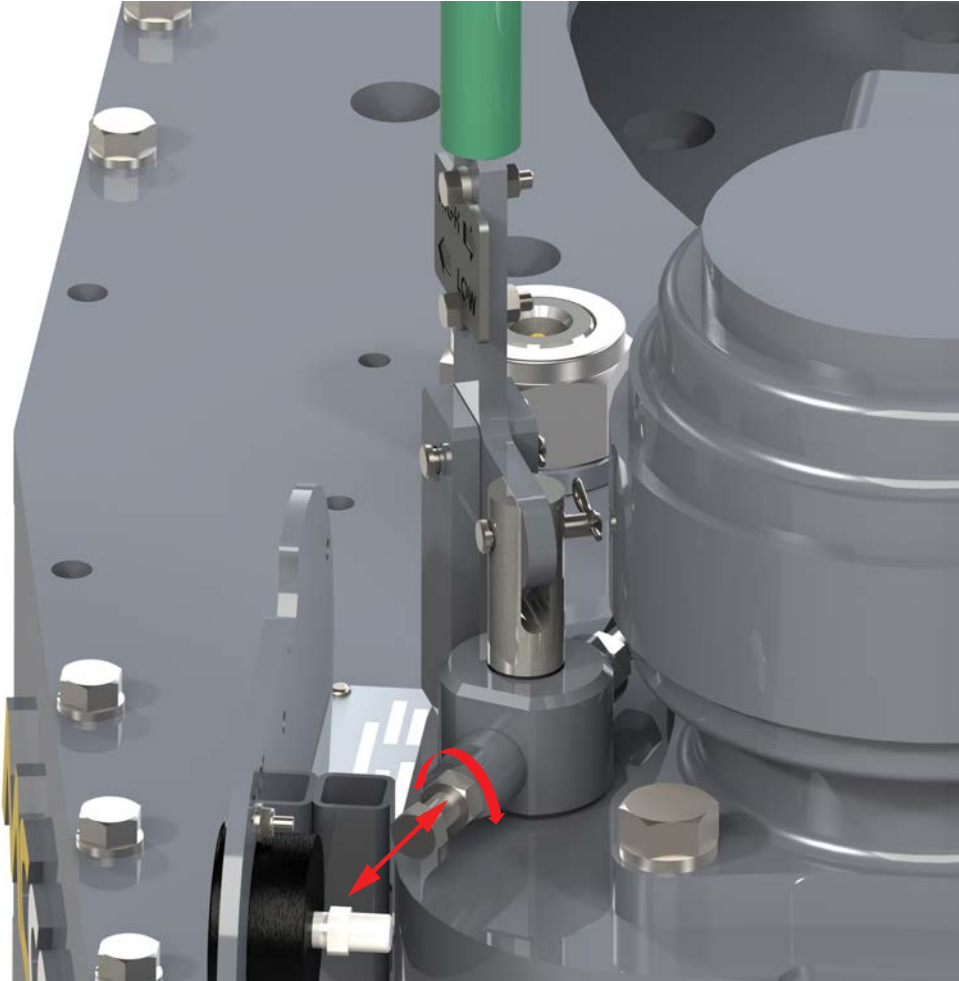
Illustration 3.F.2: Shifter Detent Force Adjustment
