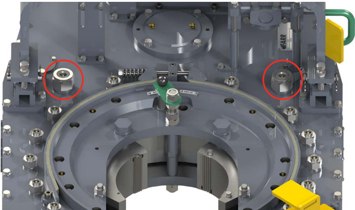
Illustration 3.E.3: Rotary Idler Lubrication
