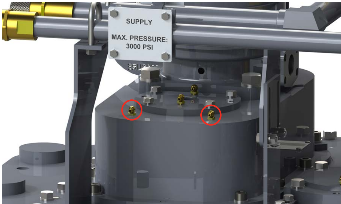
Illustration 3.E.7: Motor Mount Lubrication
