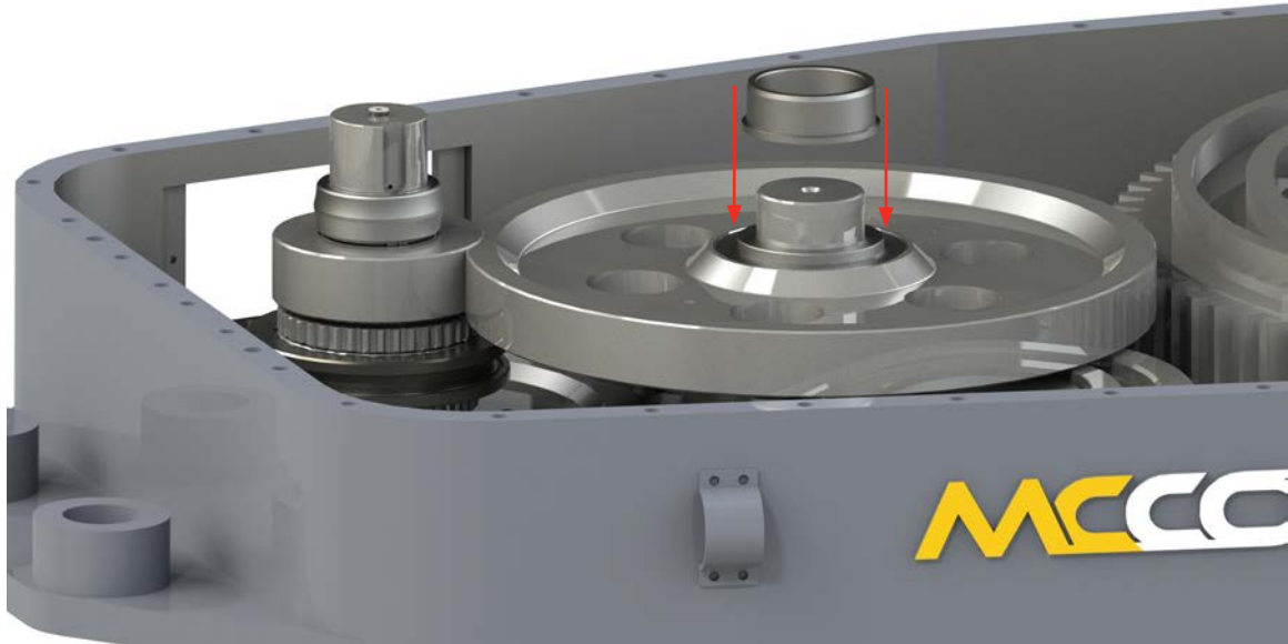
Illustration 3.1.6: Pinion Bearing Inner Race Installation
