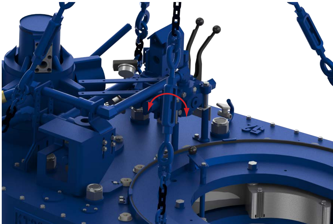
ILLUSTRATION 2.G.3: LEVELING TONG USING TURNBUCKLES
