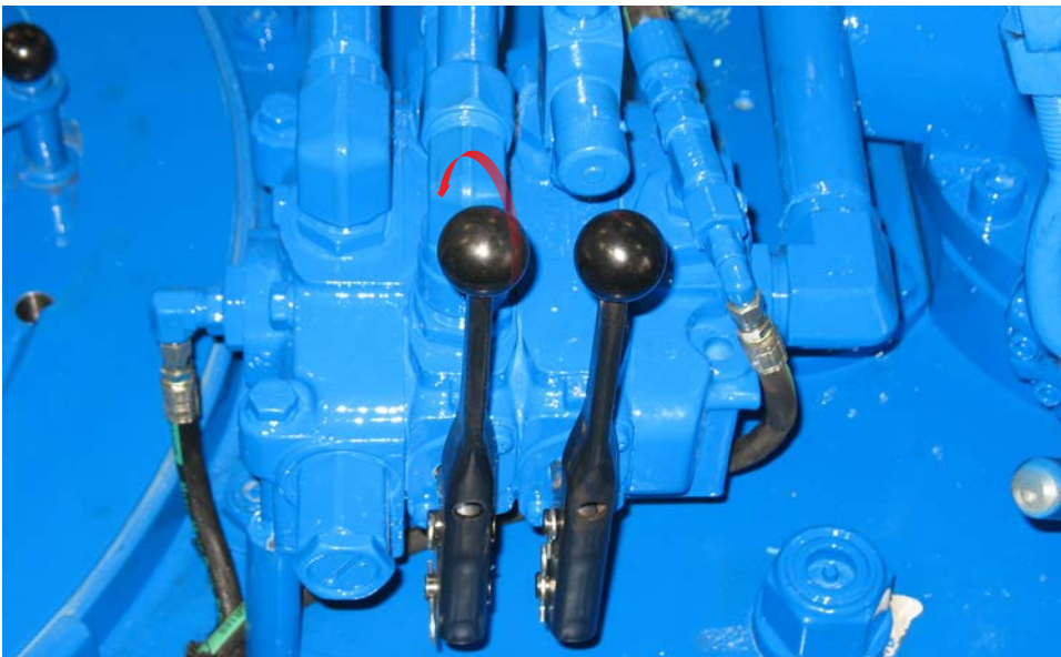
ILLUSTRATION 2.1.10: RELEASING TONG JAWS FOLLOWING BREAK-OUT & UN-THREADING
