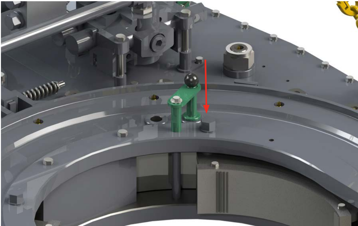
Illustration 4.1.3: Setting Backing Pin To “Break-Out” Position
