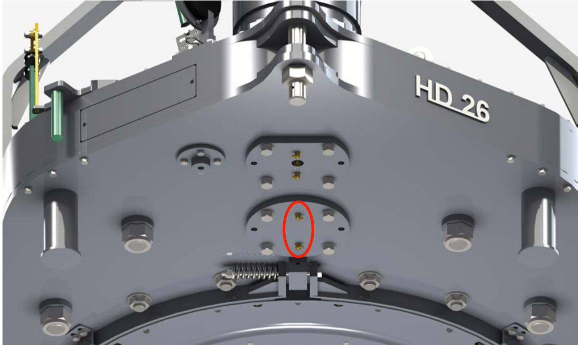
Illustration 5.5.6: Pinion Bearing Lubrication (Bottom Plate)
