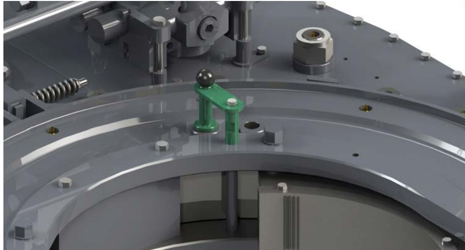
Illustration 4.1.2: Backing Pin Set To “Make-up” Position
