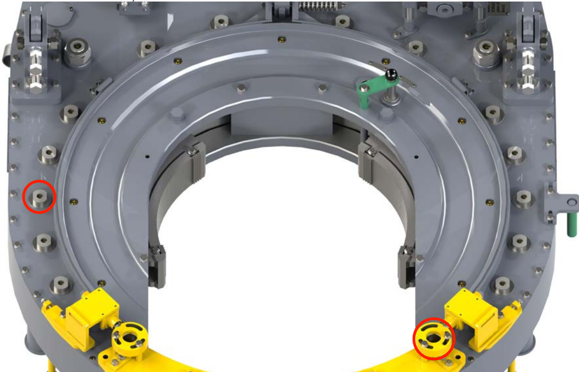
Illustration 5.5.2: Support Roller Lubrication
