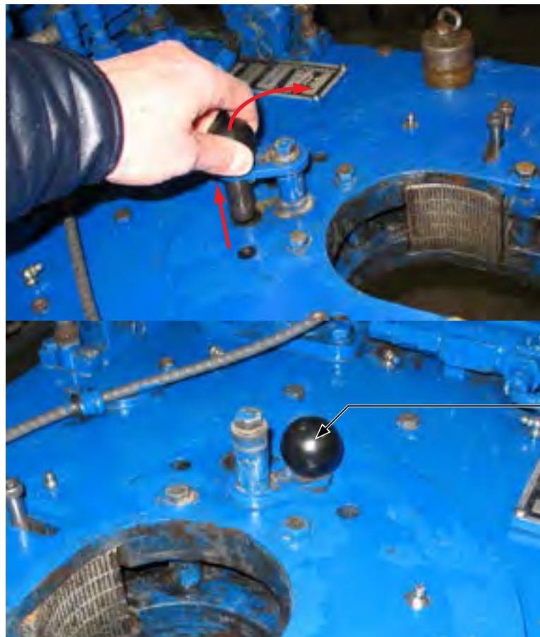
ILLUSTRATION 3.B.16: SETTING BACKING PIN TO "BREAK-OUT" MODE
