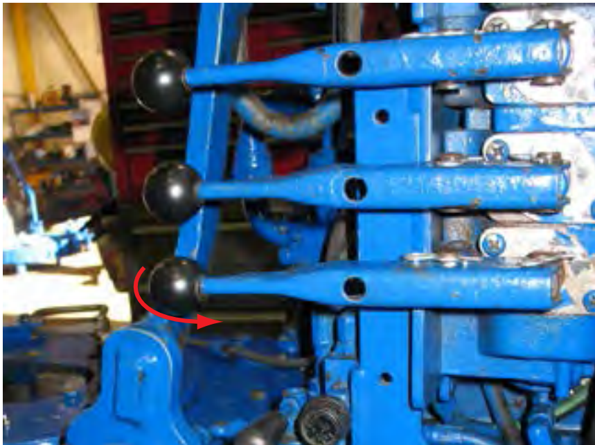
ILLUSTRATION 3.B.14: UN-CLAMPING BACKUP JAWS
