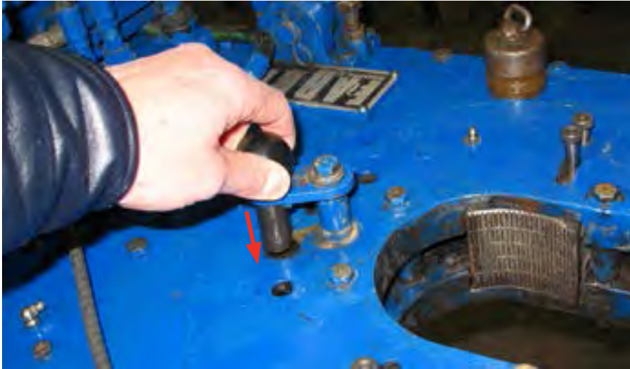
ILLUSTRATION 3.B.2: SETTING BACKING PIN TO "MAKE-UP"
