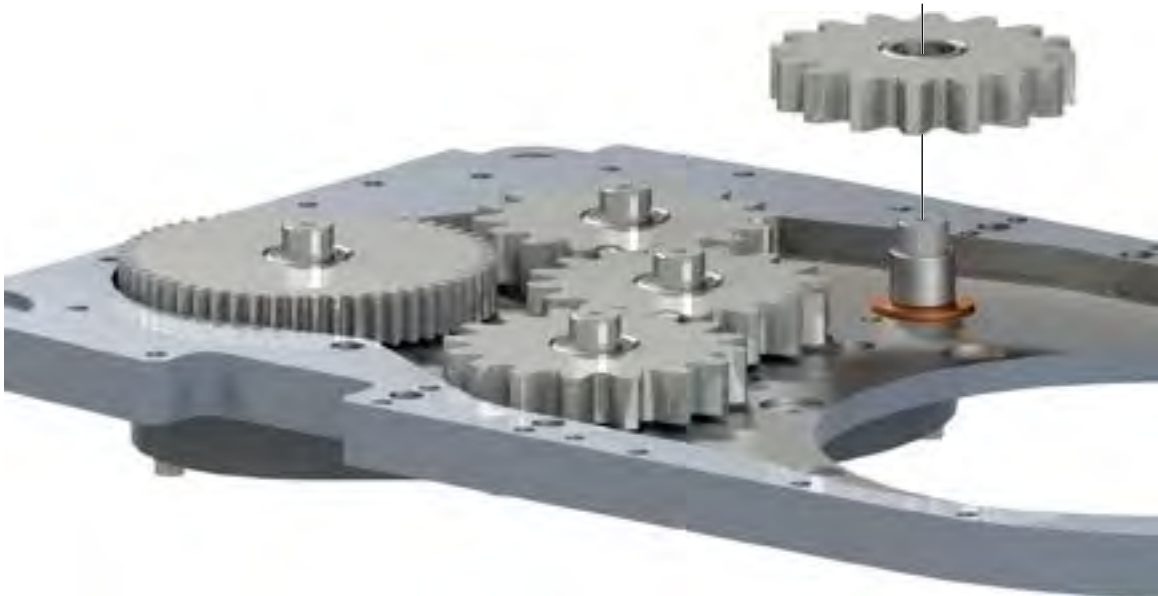
ILLUSTRATION 4.1.6: PINION GEAR INSTALLATION
