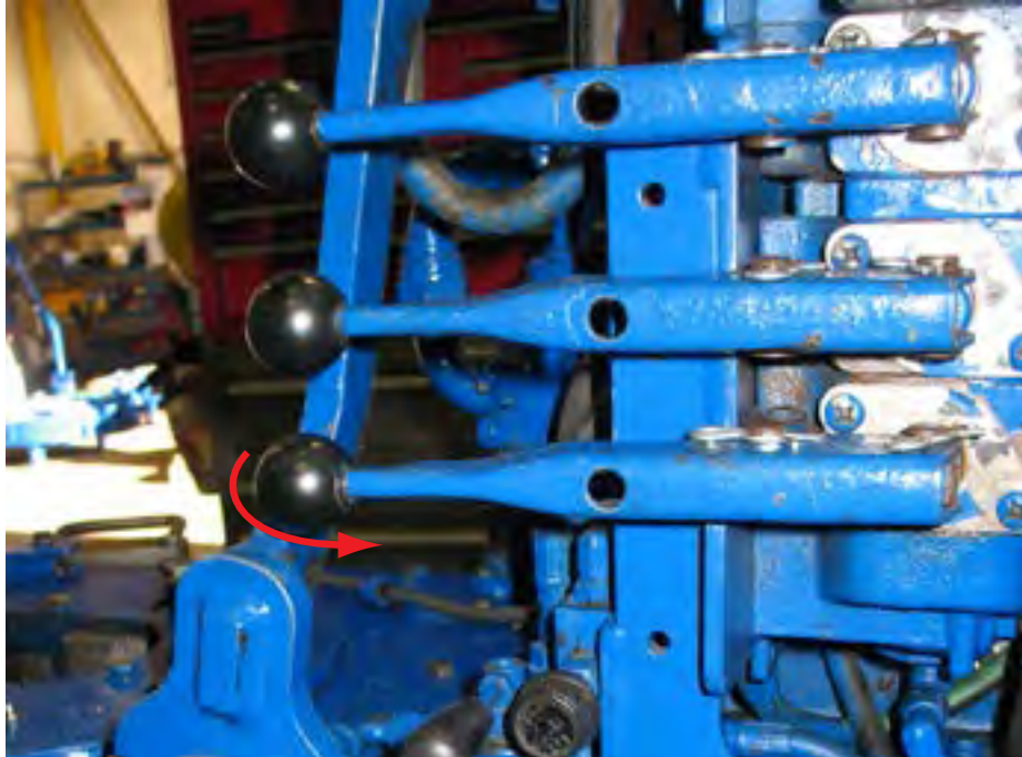
ILLUSTRATION 3.B.20: UN-CLAMPING BACKUP JAWS
