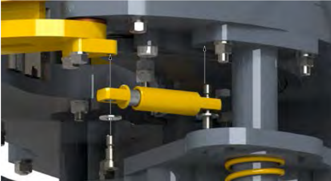
ILLUSTRATION 4.1.19: DOOR SPRING RETURN CYLINDER INSTALLATION
