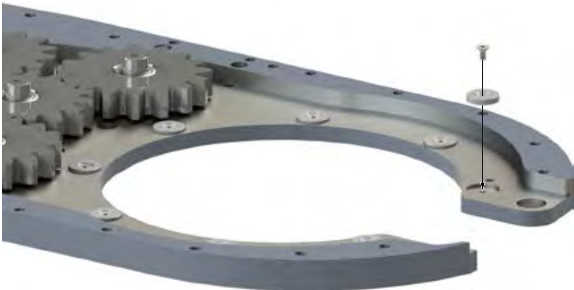
ILLUSTRATION 4.1.7: BUTTON GUIDE INSTALLATION
