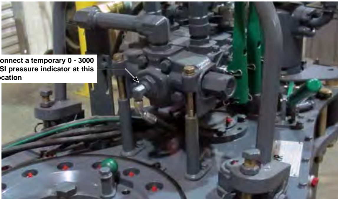
ILLUSTRATION 5.B.1: RELIEF VALVE TROUBLESHOOTING - TEMPORARY GAUGE INSTALLATION
