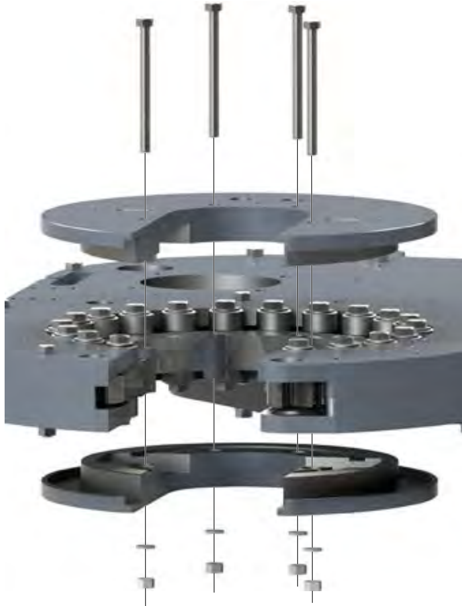
ILLUSTRATION 4.1.12: CAGE PLATE INSTALLATION
