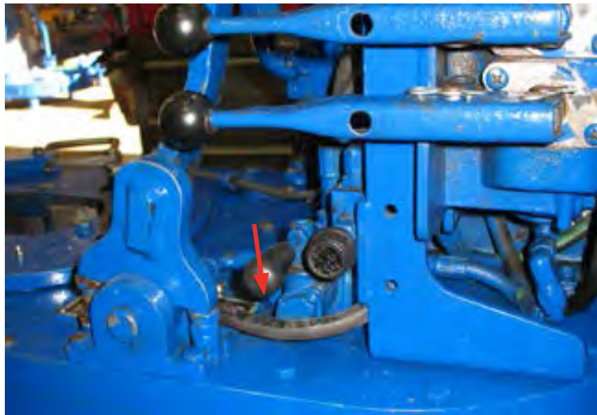
ILLUSTRATION 3.B.12: SWITCHING MOTOR SPEED SWITCH TO LOW SPEED
