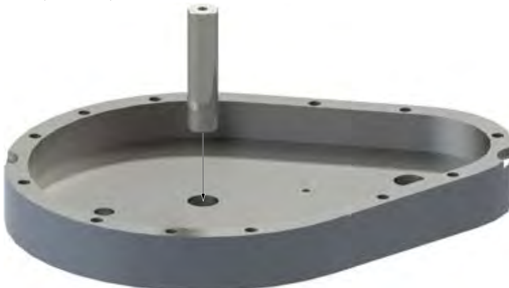
ILLUSTRATION 4.1.1: INITIAL REDUCTION GEAR SHAFT INSTALLATION
