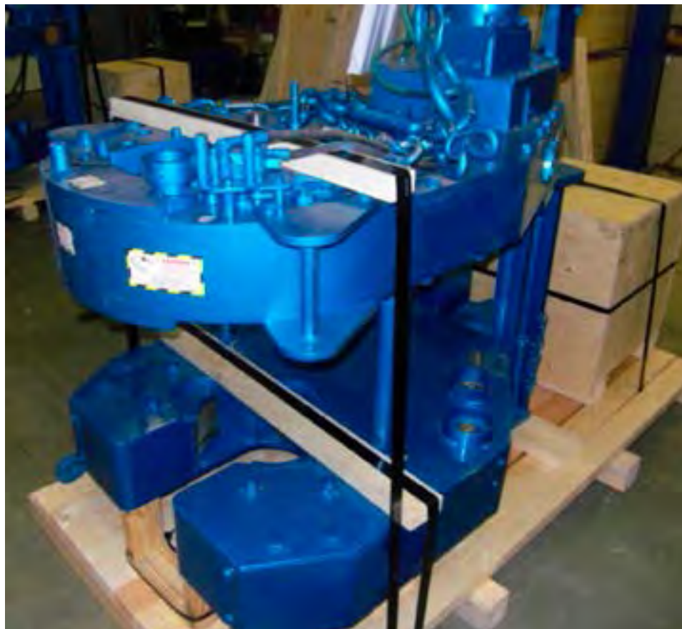
ILLUSTRATION 4.M.4: SHIPPING INSTRUCTIONS - STRAPPING EQUIPMENT TO PALLET
