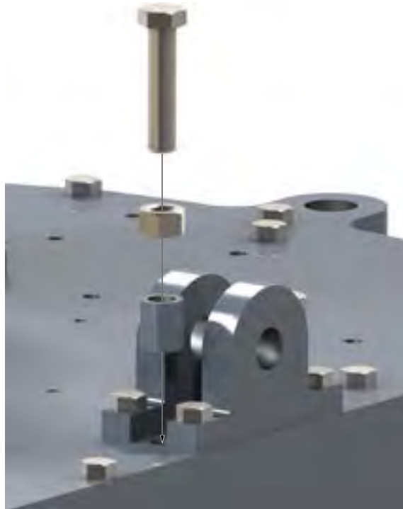
ILLUSTRATION 4.I.16: LEVELING BOLT INSTALLATION
