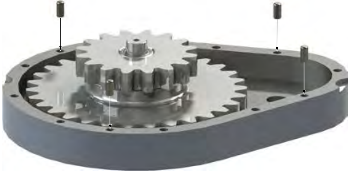
ILLUSTRATION 4.1.3: GEAR BOX COVER DOWEL PIN INSTALLATION
