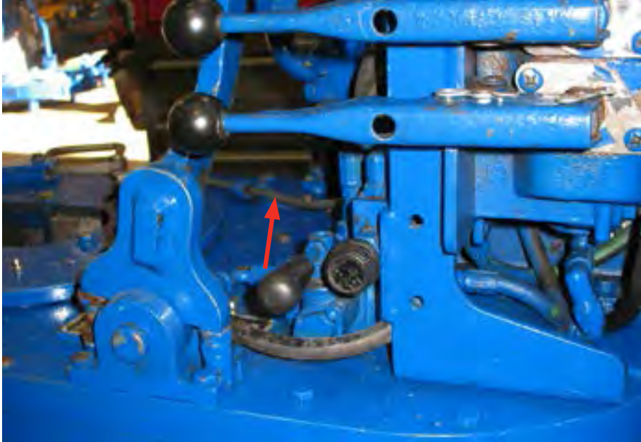
ILLUSTRATION 3.B.18: SWITCHING MOTOR SPEED CONTROL TO HIGH SPEED
