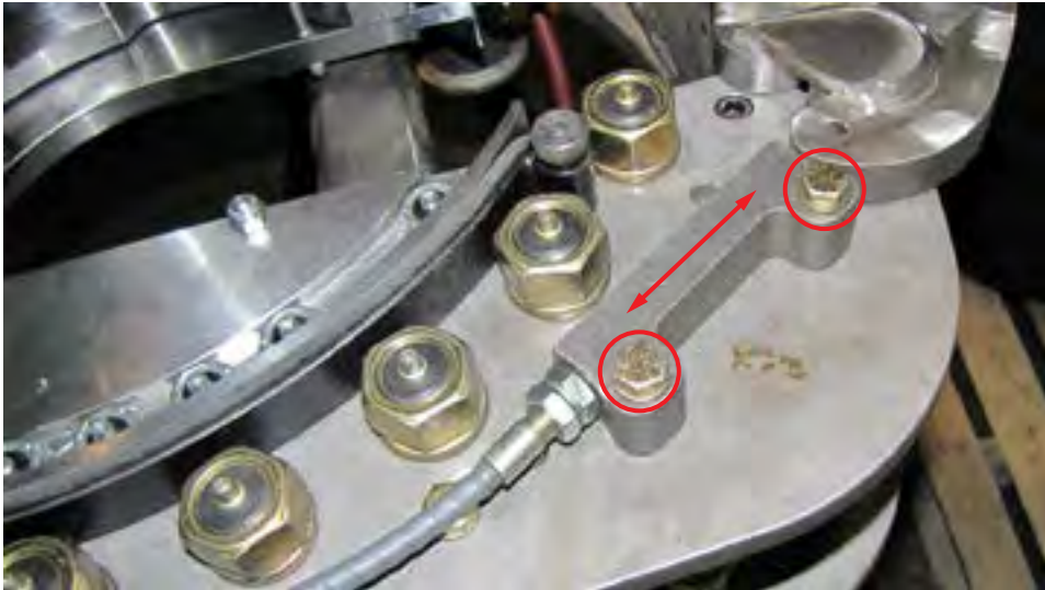
ILLUSTRATION 4.F.7: SAFETY DOOR PLUNGER ADJUSTMENT 03
