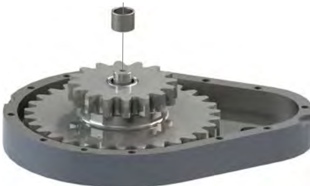
ILLUSTRATION 4.1.2: REDUCTION GEAR ASSEMBLY INSTALLATION
