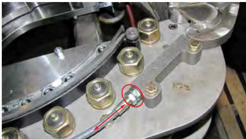
ILLUSTRATION 4.F.6: SAFETY DOOR PLUNGER ADJUSTMENT 02
