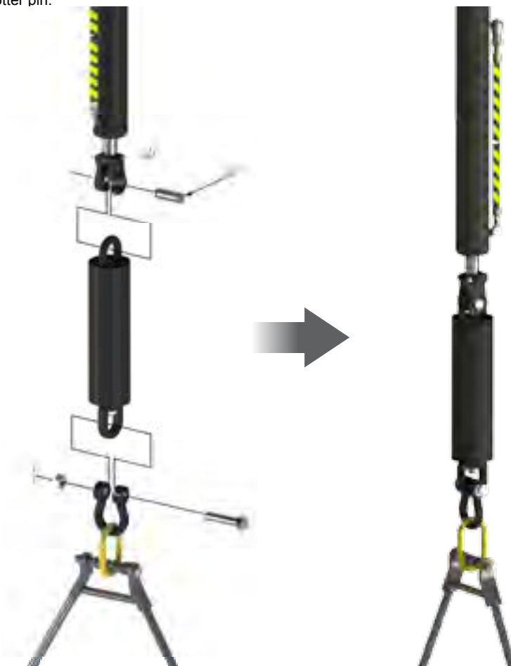
ILLUSTRATION 2.D.1: LIFT CYLINDER & SPRING HANGER INSTALLATION
