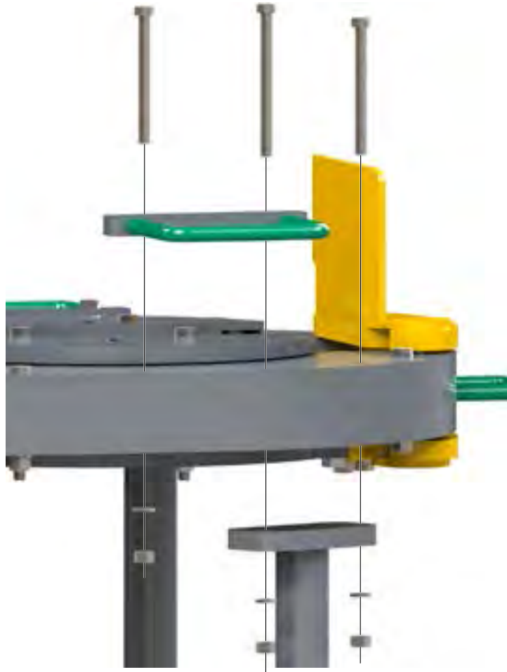
ILLUSTRATION 4.1.19: FRONT LEG WELDMENT INSTALLATION
