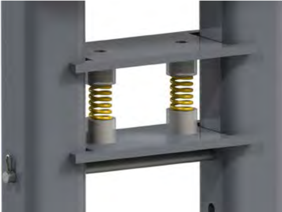
ILLUSTRATION 4.I.17: REAR BACKUP SUPPORT INSTALLATION
