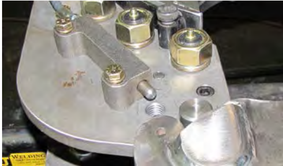
ILLUSTRATION 4.F.5: SAFETY DOOR PLUNGER ADJUSTMENT 01
