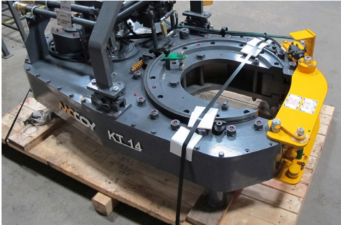
Illustration 5.10.1: Shipping Instructions - Strapping to Pallet
