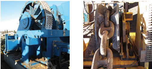
McCoy load pins and payout sensors installed in an anchor winch system.
