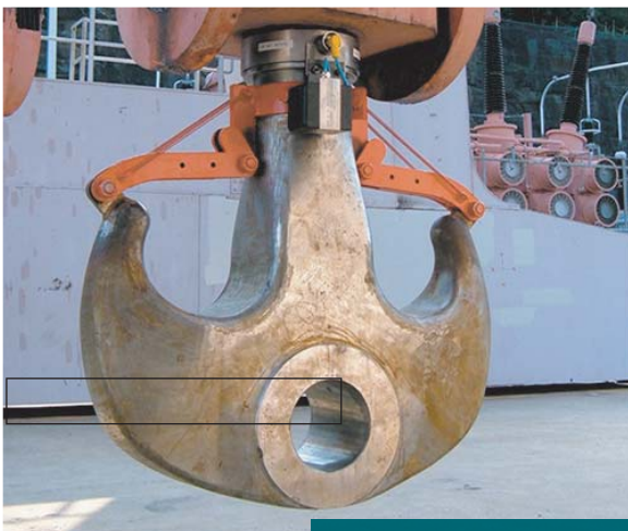
255 ton hooks with transmitters.
