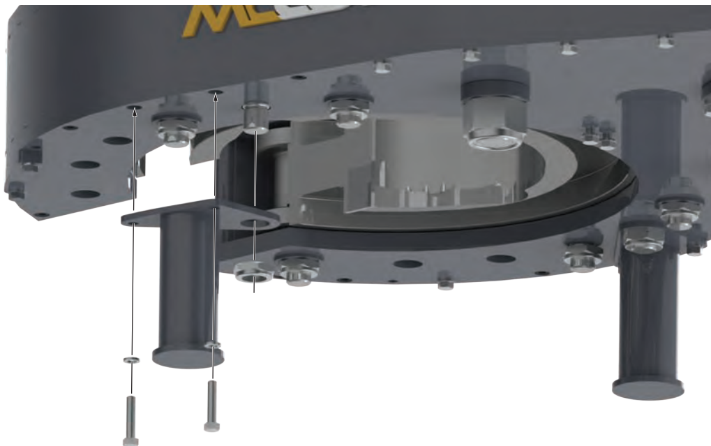
ILLUSTRATION 3.H.5: TONG ASSEMBLY - FRONT LEG INSTALLATION
