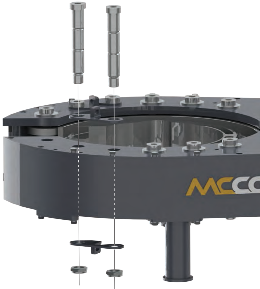
ILLUSTRATION 3.H.6: TONG ASSEMBLY - SUPPORT ROLLERS (BRAKE BAND WELDMENTS)
