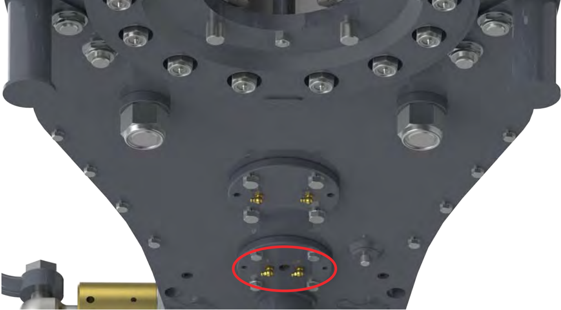
ILLUSTRATION 3.D.6: CLUTCH LUBRICATION POINTS
