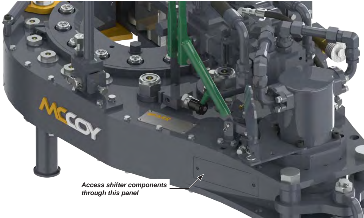
ILLUSTRATION 3.D.8: SHIFTER SHAFT LUBRICATION
