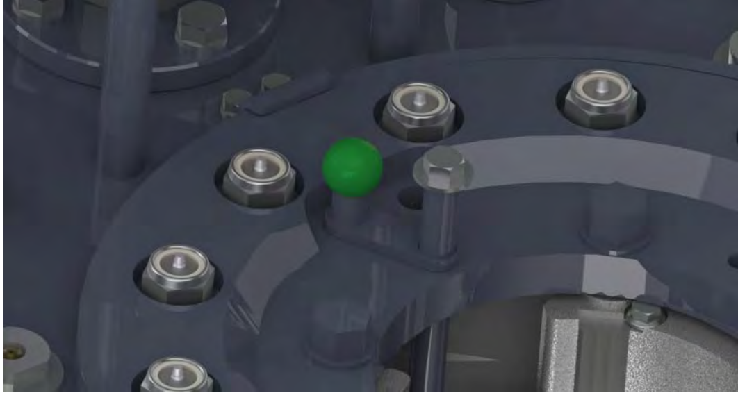
ILLUSTRATION 2.H.2: BACKING PIN SET TO "MAKE-UP" POSITION
