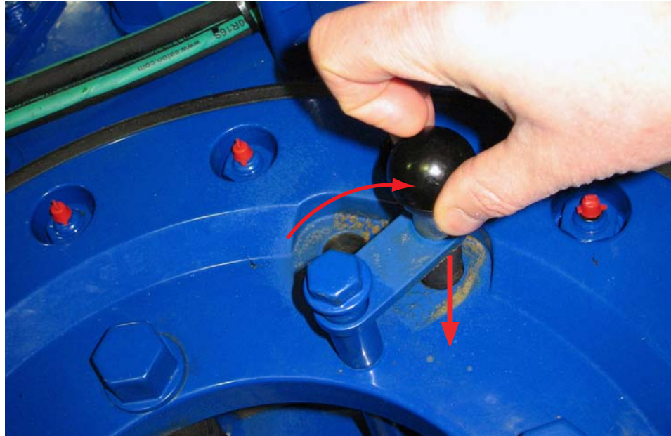
ILLUSTRATION 2.H.8: SETTING BACKING PIN TO "BREAK-OUT" POSITION
