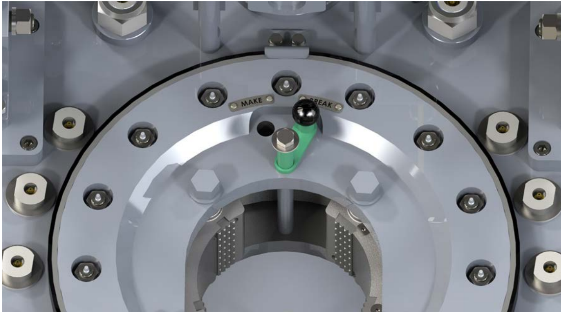
Illustration 4.1.3: Backing Pin Set To “Break-Out” Position
