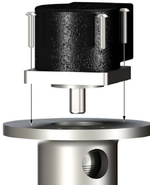
Illustration 8.1.3: Securing Encoder To Encoder Mount
