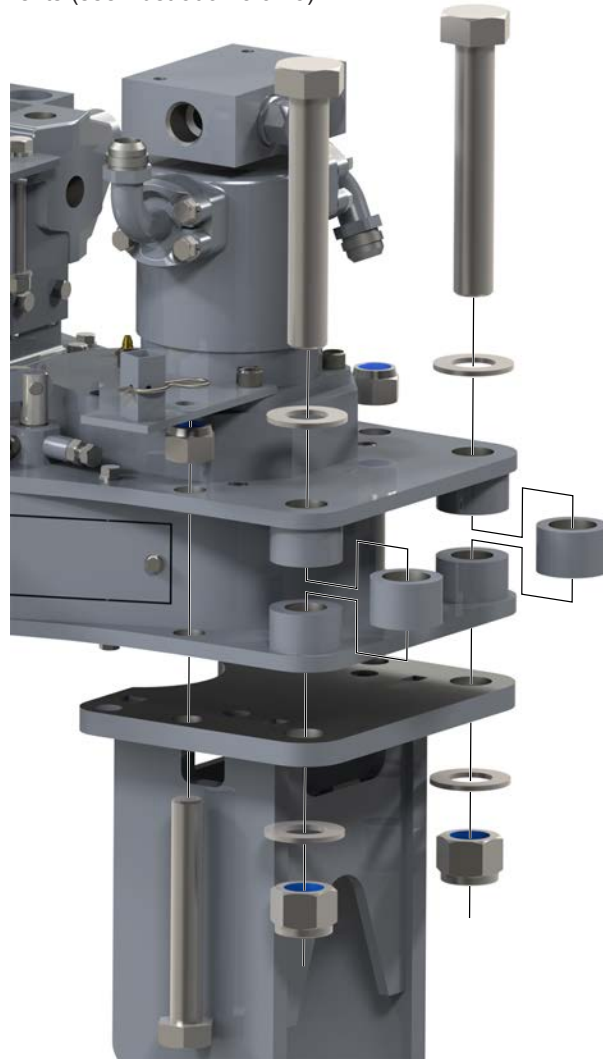
Illustration 5.9.13: Tong Assembly - Rear Leg Installation
