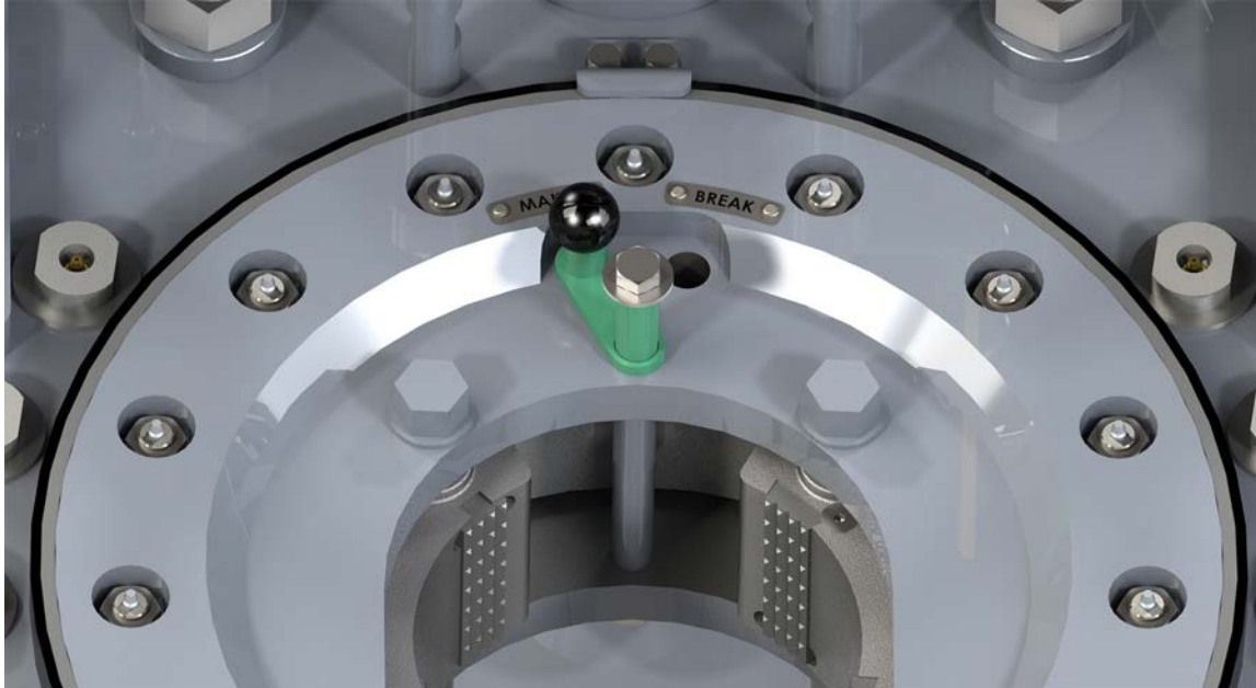
Illustration 4.1.2: Setting Backing Pin To “Make-up” Position
