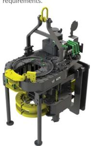
As an option, we offer the most reliable in the industry Lockjaw Style Backup. With its three jaws technology, the Lockjaw Backup provides exceptional gripping capabilities with reduced pipe deformation, stress, and marking. The Backup offers a gripping range from 4-1/2" through 11-3/4" (114 mm to 298.5 mm).
