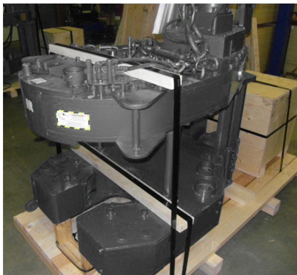
Illustration 5.10.1: Shipping Instructions - Strapping Equipment To Pallet
